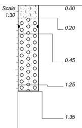
Slightly moist, pale brown, very loose, silty SAND. Topsoil.
