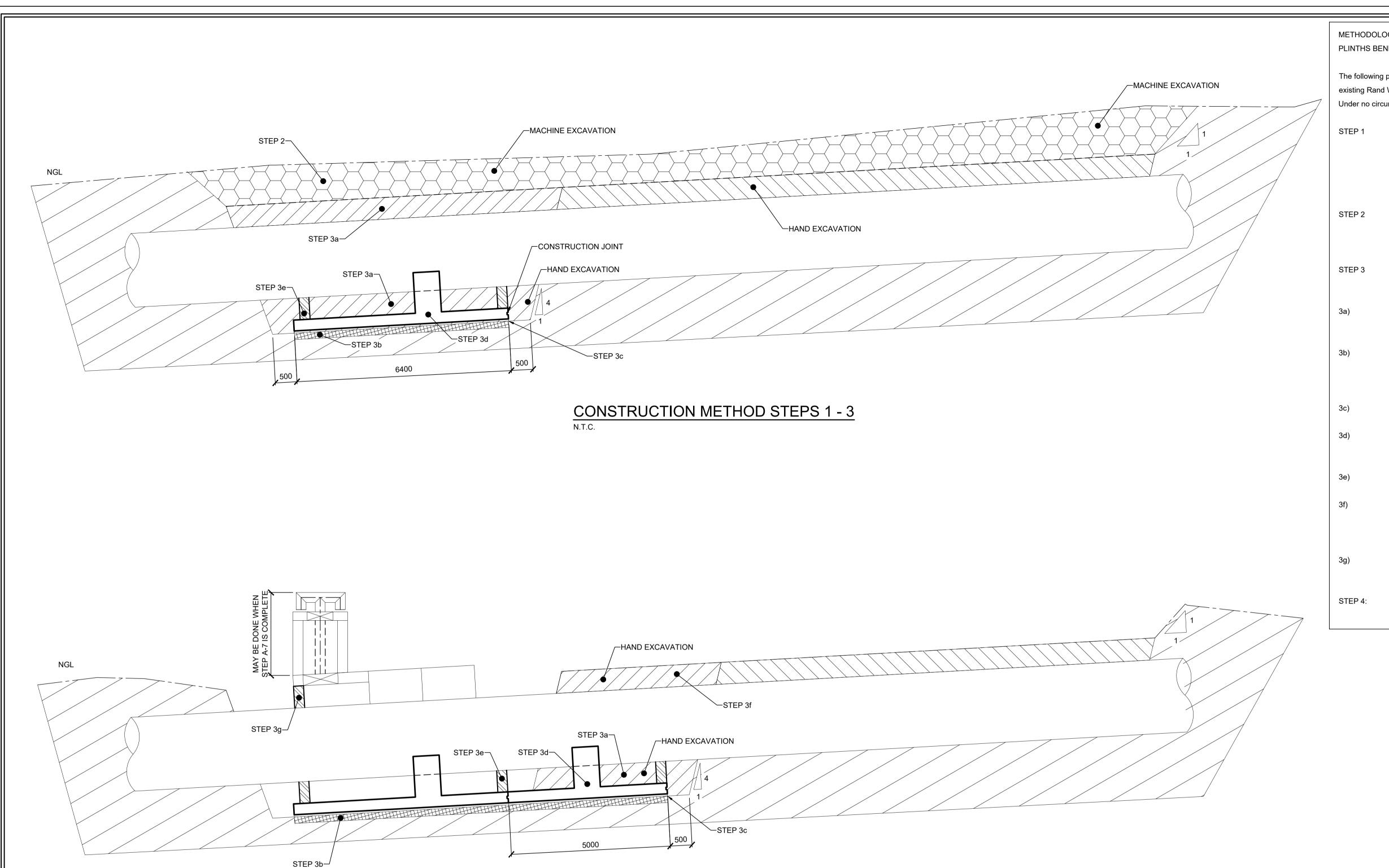
CONSTRUCTION METHOD SEQUENTIAL REPETITION OF STEPS 1 - 3
