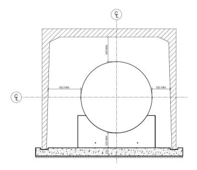
In all cases where precast concrete culverts are prescribed, it is specified that such culverts are to comply with SANS 986. Using the prescribed testing method and proof loads as given in SANS 986, a verification will be made in Section 4: Analysis and Detail Design Calculations to verify that the anticipated loads at positions in which the precast culverts are specified are less than or equal to the proof loads as stated. In the current case, a specification of 75S is specified.
