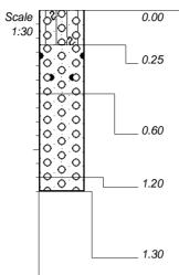
Moist, orange brown, loose, sandy silt with GRAVEL. Topsoil with abundant fine roots.
